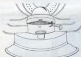
Showing Double Bayonet Burner Lock.
