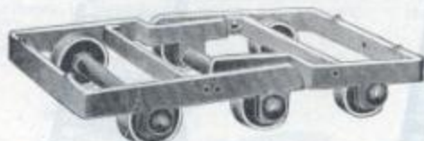
Steel Frame, Flexible.
