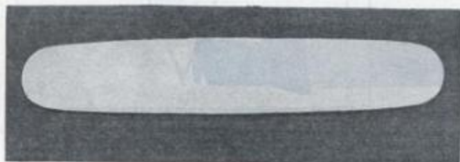
No. 8—Sheet Brass, from which Linings are Pressed.
