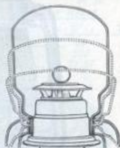
Showing Device for Holding Handle in any Desired Position on Cold Blast Lanterns.
