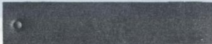
No. 12—Brass Strip, Pierced, Ready to Receive Bolster.
