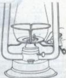
Showing Lifting Device on Cold Blast Lanterns.
